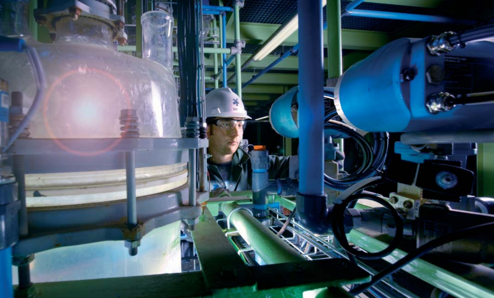
Herman du Preez conducting operational maintenance on a glass cooling tower experimental system that evaluates alternative sources of cooling water to minimise fresh water intake.
