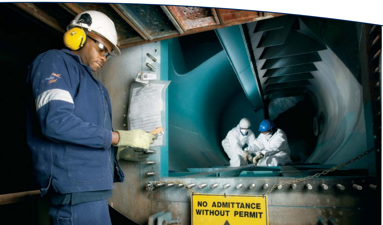
Lucas Mngomezulu, production standby, checking for the possible presence of gases in a vessel that requires special safety measures for confined space entry.
